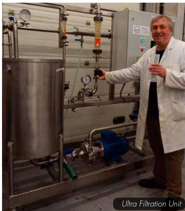
processes is the use of membrane filtration to separate out various fractions that are produced as a result of enzymatic hydrolysis. To do this a pilot scale ultrafiltration unit, supplied by Axium Process Ltd, which can separate out materials with well defined molecular weight ranges has been installed in line.
