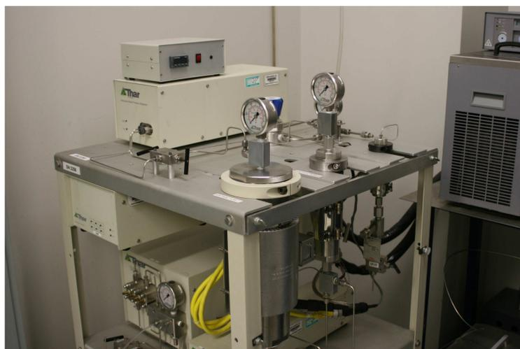
Figure 3. Thar CO<sub>2</sub> extraction unit
